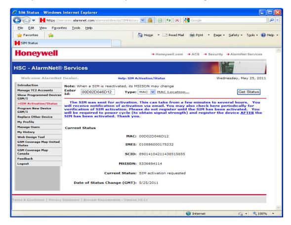
After you receive the email confirming SIM activation, sample shown below, power-cycle the radio to obtain signal strength and complete the activation process.
